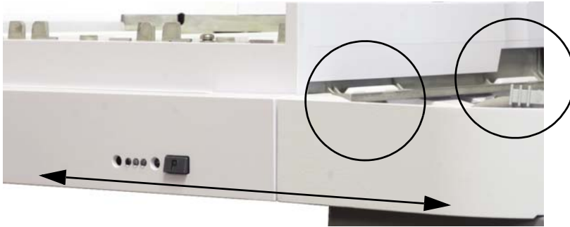
Figure 5 Sample tray correctly installed.
