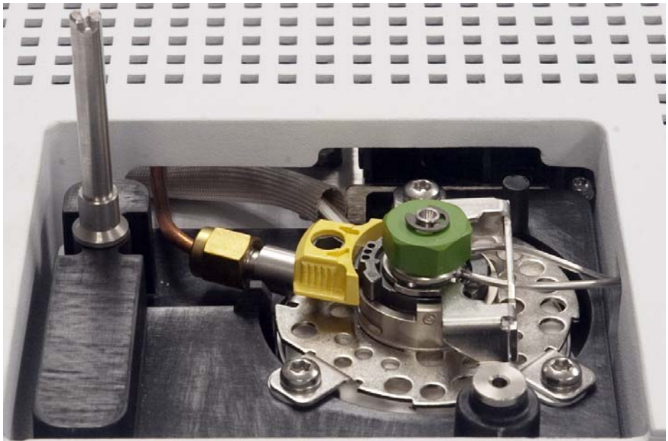
Figure 14 Installing the mounting post (5975T LTM-GC/MSD)
