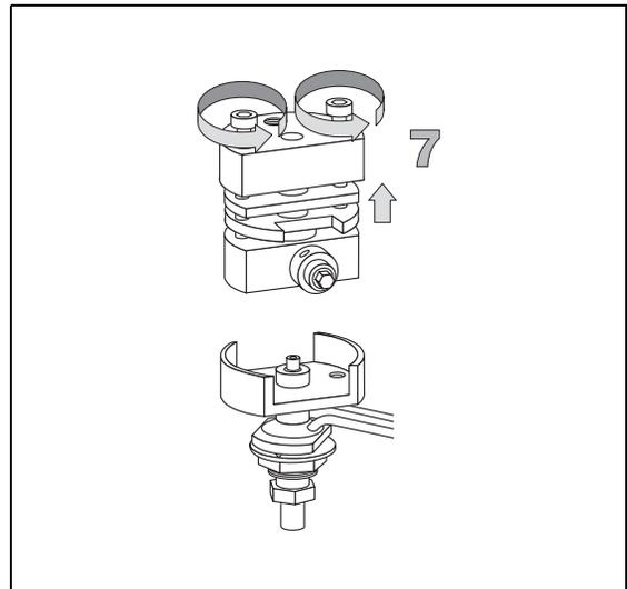
8. Disassemble the injector body, separating the head from the lower part.
