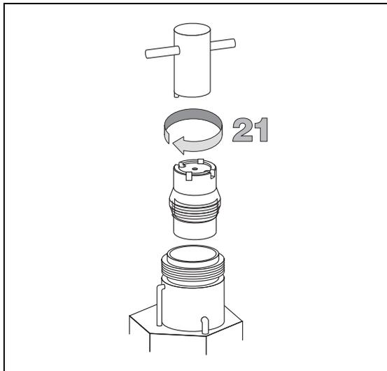
22. Place the septum holder with the septum onto the inlet port, then screw and tighten the ring nut up to the stop.
