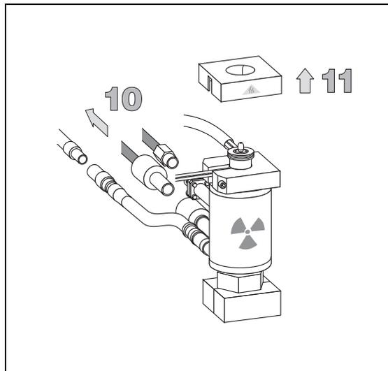
12. Remove the heater from the top of the ECD detector unscrewing and removing the 4 mm Allen fixing screw. Use a 3 mm Allen wrench.
