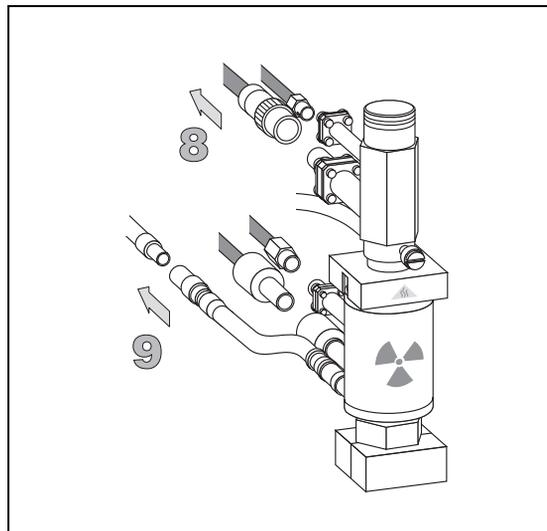
10. Loosen the nut that fixes the ECD detector to its base body with the proper tool contained in the standard outfit and remove the detectors from the ECD base body.
