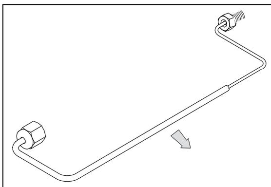
11. Connect the new split line tubing to the injector body.
