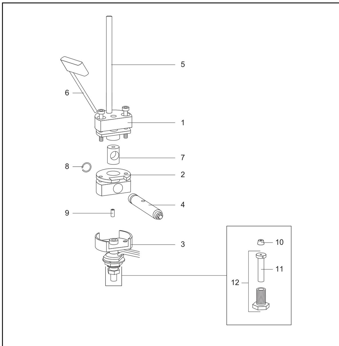
**Table 6-1.** Manual Cold On-Column Injector parts identification table
