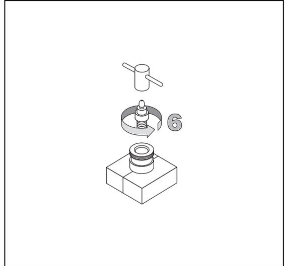
7. Place a new jet into its housing and tighten it with the proper tool.
