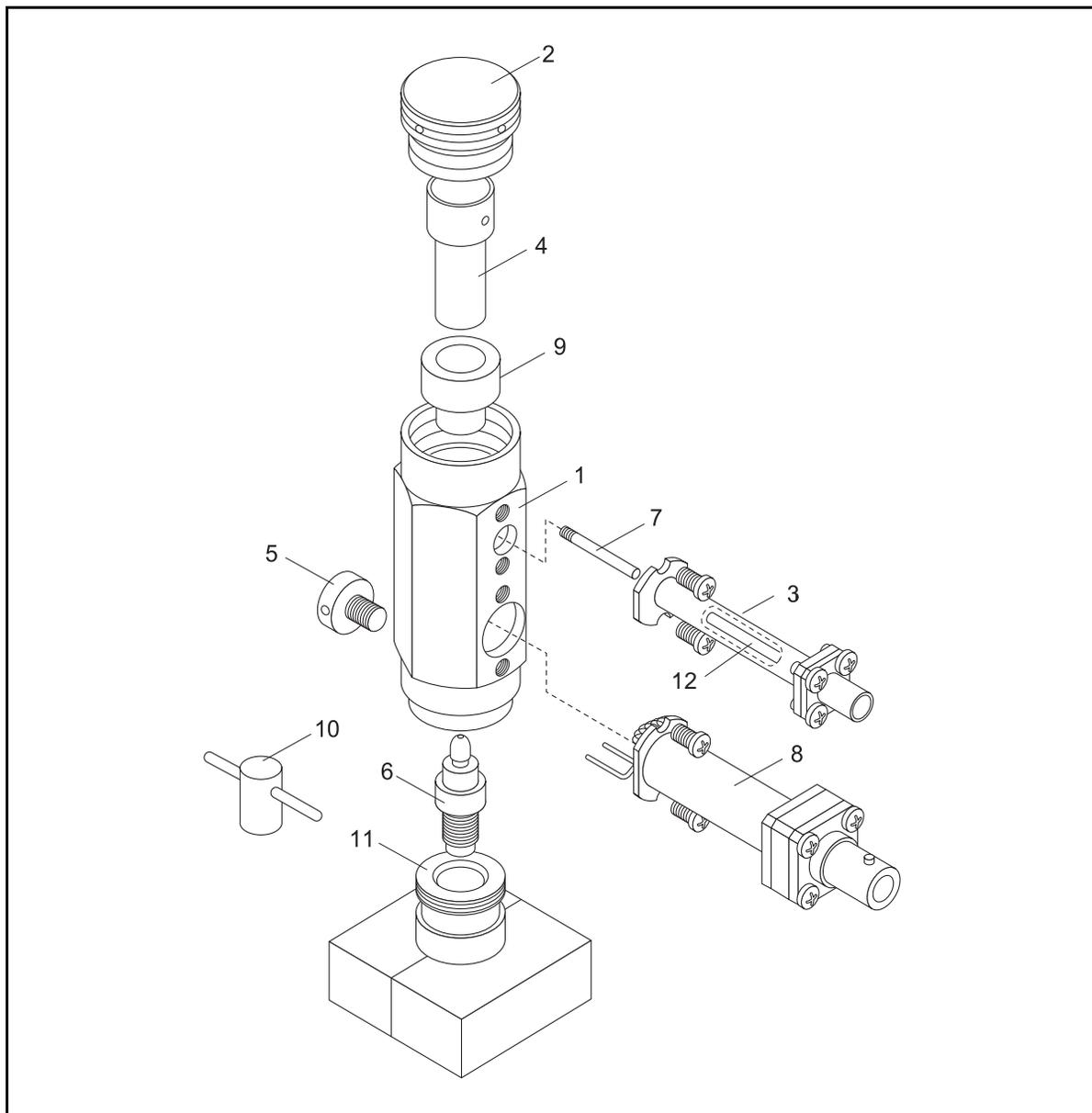
**Table 11-1.** Flame Ionization Detector (FID) parts identification table
