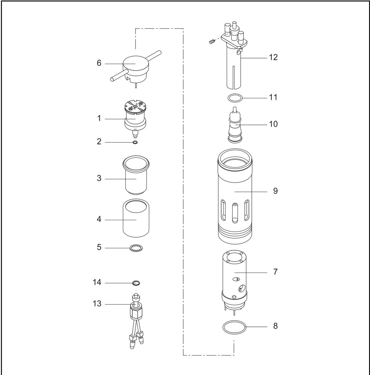
**Table 15-1.** Photoionization Detector (PID) parts identification table
