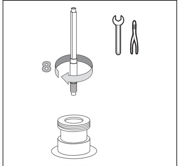
9. Place the detector on its base body, paying attention that the aluminium ring has been inserted in the correct position, then tighten the fixing nut.
