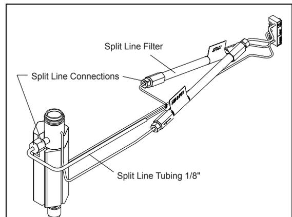
11. Connect the new split line tubing to the injector body.
