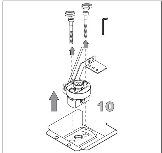
11. Disassemble the injector body, separating the head from the lower part.
