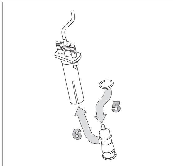
7. Insert the lamp holder into the lamp housing
