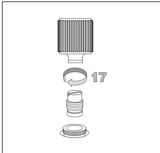
18. Insert the analytical column with its ferrule into the bottom of the injector in its previous position. Refer to the TRACE™ GC Operating Manual for instructions.
