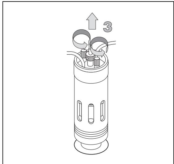
4. Remove the lamp with its Viton™ O-ring from the lamp holder.
