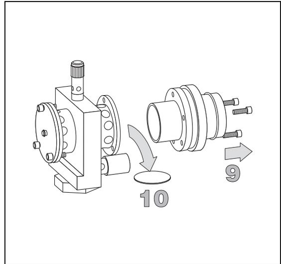
11. If you want to replace only the filter-side heat shield, go to # 21. If you want to replace the flame-side heat shield, loosen the three Allen screws that fix the flange to the detector body and remove it with the spacer that should remain inserted in the flange. Now you could access the flame-side heat shield and the relevant graphite seal.
