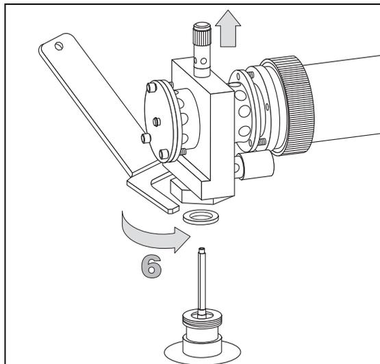
7. Using the 5 mm wrench provided with the GC, loosen the jet and remove it from the detector base body.
