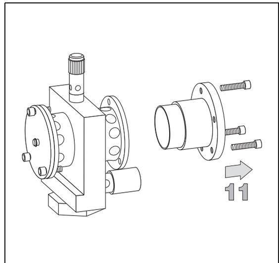
12. Loosen the Allen screws that fix the mirror plug and remove it.
