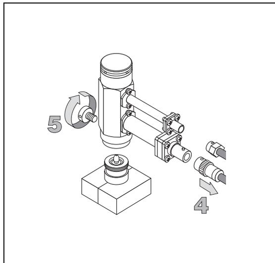
6. Unscrew the two fixing screws and remove the lower connector holder assembly from the detector cell.
