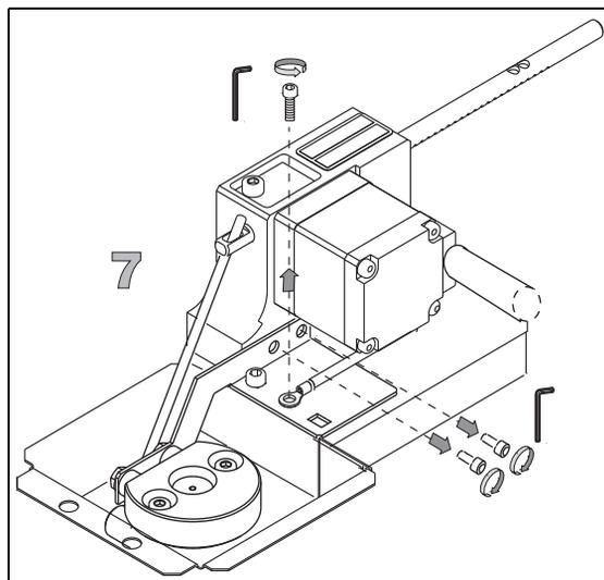
8. Move vertically the valve lever to allows its extraction through the slot on the actuator shaft. Carefully lift up the automatic actuator to remove it from the OC housing.
