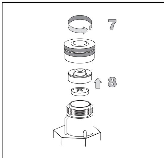
9. Use the liner cap wrench provided with the GC to remove the injector liner cap.
