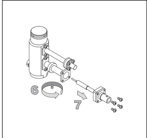
8. Gently replace the thermionic source, pushing it in straight.
