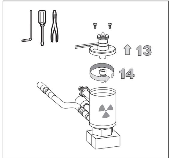
15. If you are going to replace the collecting electrode with a new one, go to step 16. If you are going to clean it, put it into an ultrasonic bath filled with a toluene/hexane mixture and sonicate it. In the most critical cases, fine emery paper can be used.
