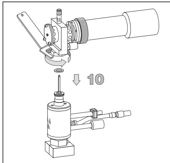
11. Reconnect the excitation and heater cables to the ECD detector.
