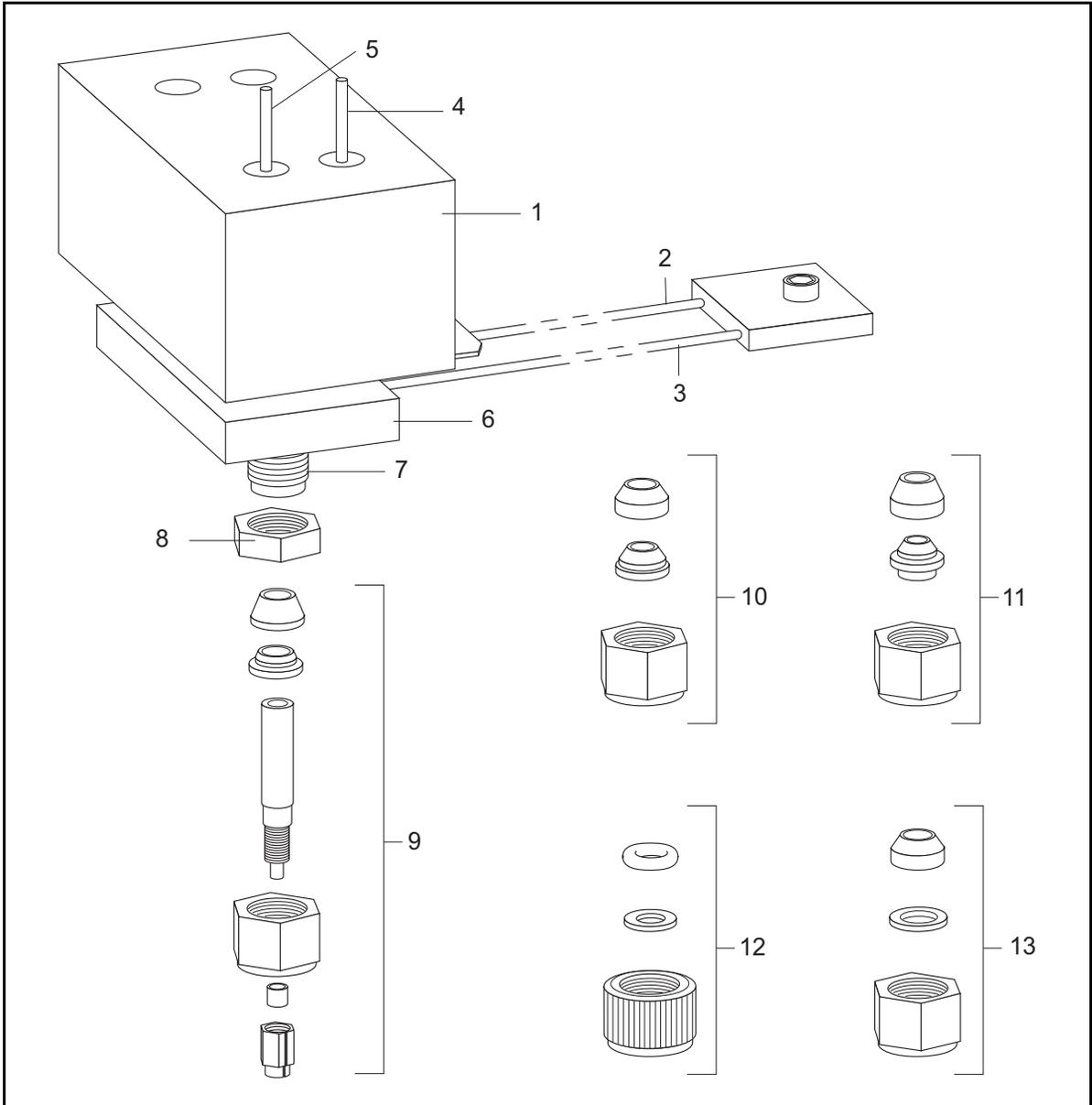
**Table 16-1.** Thermal Conductivity Detector (TCD) parts identification table
