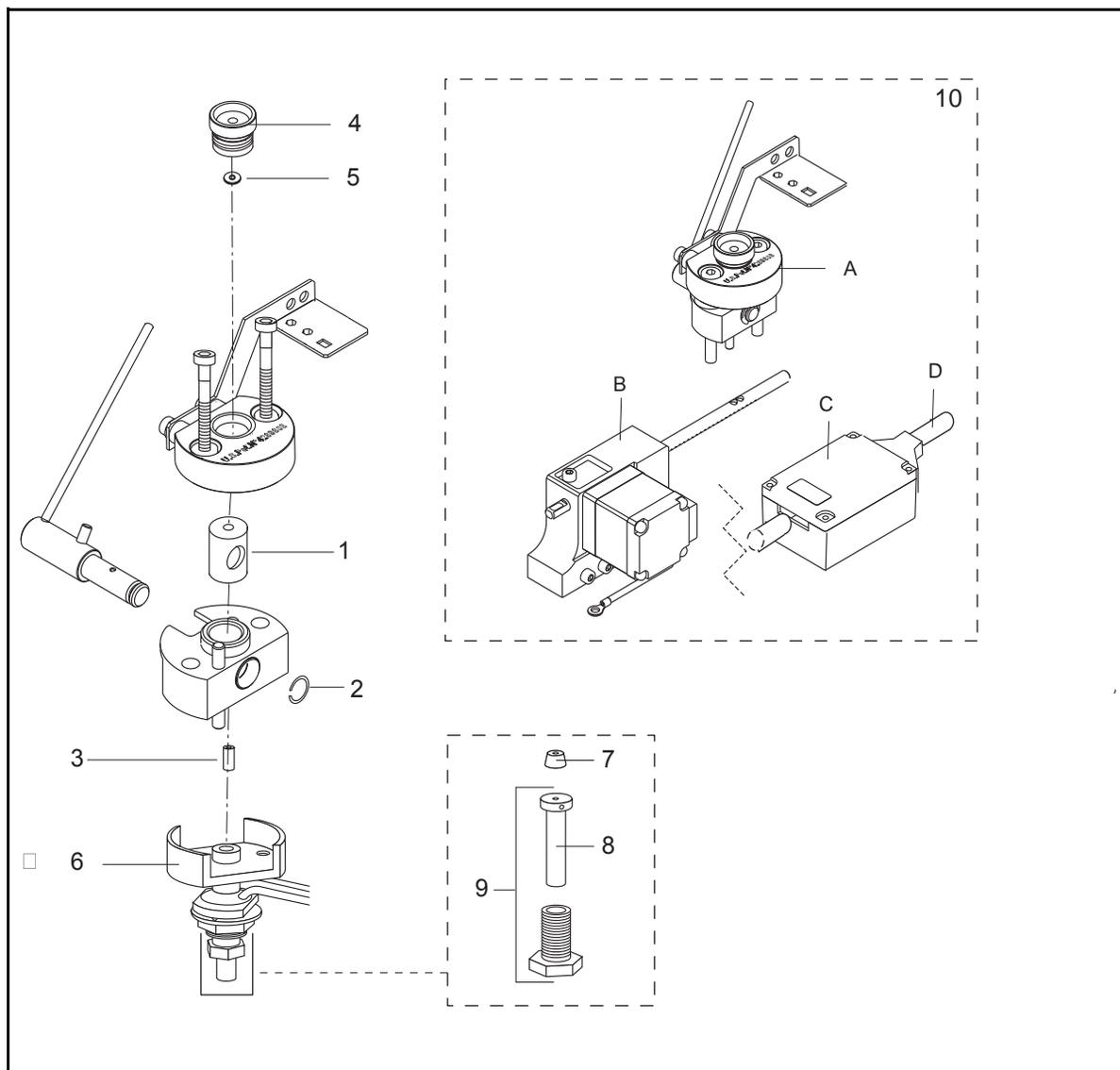
**Table 4-1.** Automated Operation Cold On-Column Injector Parts Identification Table
