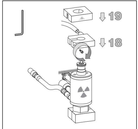
20. Remount the NPD detector on the top of the ECD and tighten the fixing screw.
