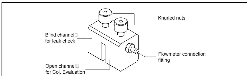
Figure 10-1. Column-flow Meter Connector
