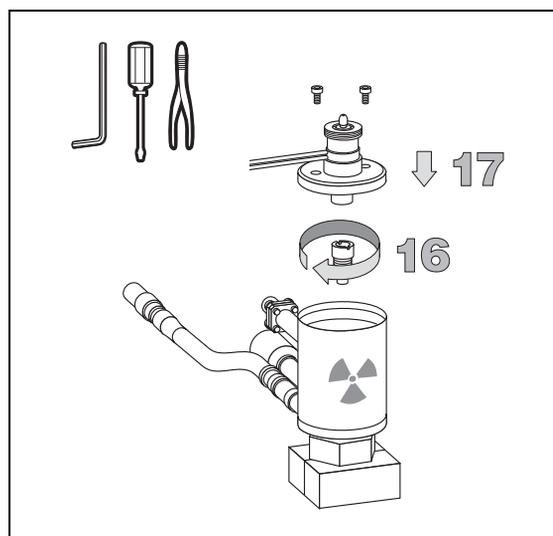
18. Reinsert the heater on the top of the ECD detector and fix it with its Allen screw.
