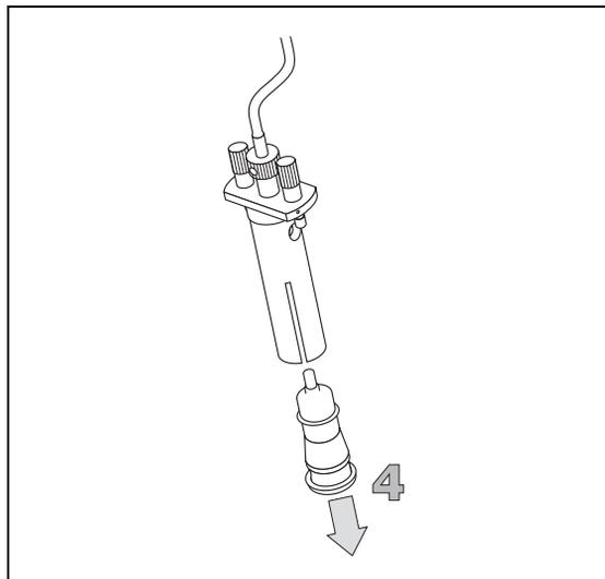
5. Remove the Viton™ O-ring from the lamp.
