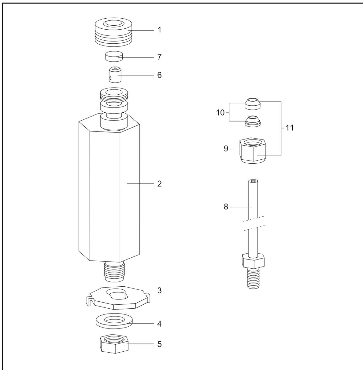
**Table 7-1.** Packed Column Injector parts identification table
