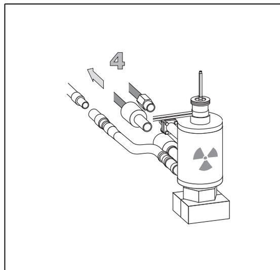
5. Remove the detector adapter unscrewing the two retaining Allen screws. Use a 2.5 mm Allen wrench.
