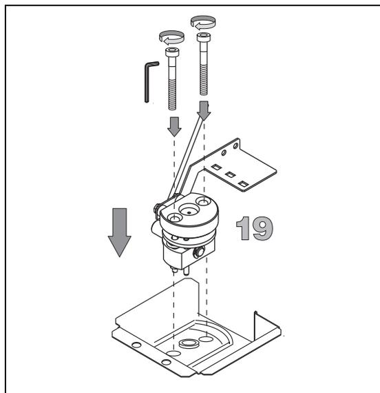
20. Fix the OC head on the ceiling of the GC and tighten the two screws A on the side of the OC head previously loosened.
