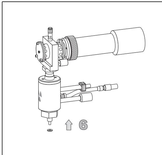
7. Remount the detectors on the ECD base body, tightening the fixing nut with the proper tool.
