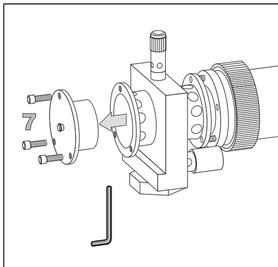
10. Insert the mirror plug in the detector body and fix it with the relevant Allen screws.
