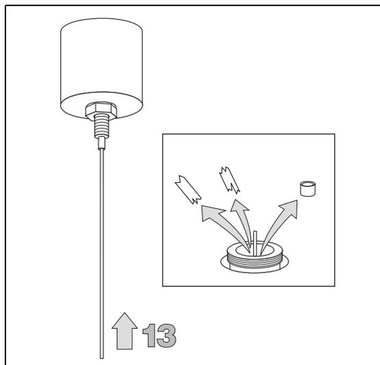
14. Use tweezers to reinsert the spacer inside the injector, complying with the correct orientation.
