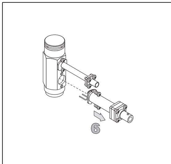
7. Remount the new connector holder assembly and fix it to the detector cell using the two screws. Make sure the connecting fork is placed downwards to achieve the correct contact with the jet.
