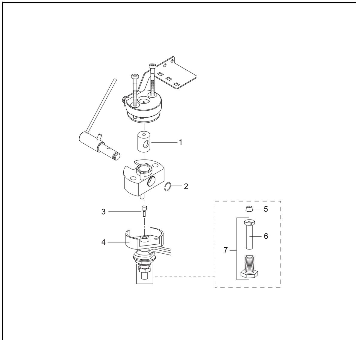
**Table 5-1.** Automated Operation Cold On-Column Injector parts identification table
