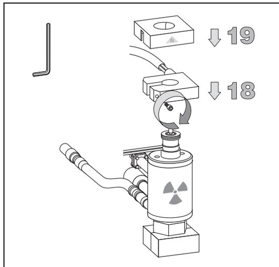
20. Remount the FID detector on the top of the ECD and tighten the fixing screw.
