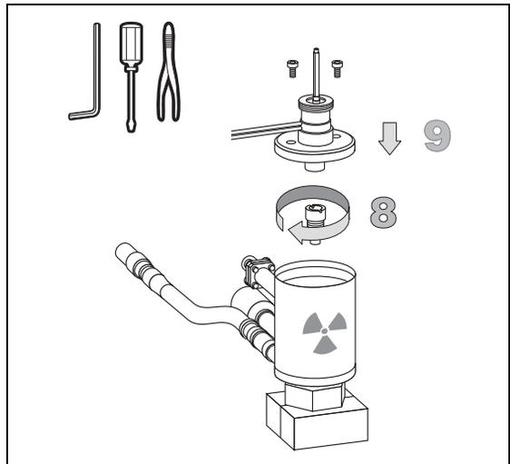
10. Place the FPD detector on the ECD top cover, paying attention that the aluminium ring has been inserted in the correct position, then tighten the fixing nut.
