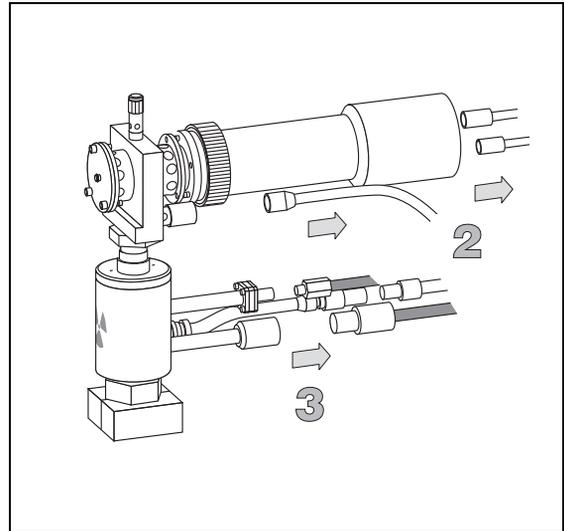
4. Loosen the nut that fixes the ECD detector to its base body with the proper tool contained in the standard outfit and remove the detectors from the ECD base body.
