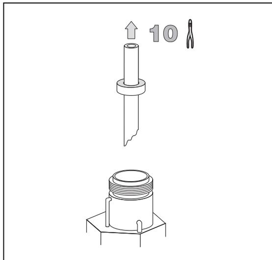
11. Unscrew the nut that retains the analytical column.
