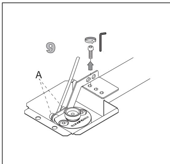
10. Unscrew the two Allen bolts that fix the injector body to the injector base. Remove the injector body from its base.
