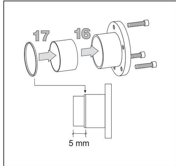
18. Insert the flange into the detector body and fix it tightening the three Allen screws.
