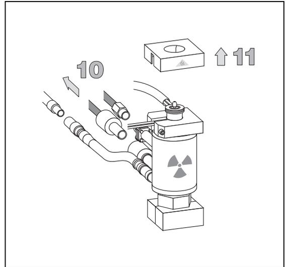
12. Remove the heater from the top of the ECD detector loosening the Allen fixing screw. Use a 3 mm Allen wrench.
