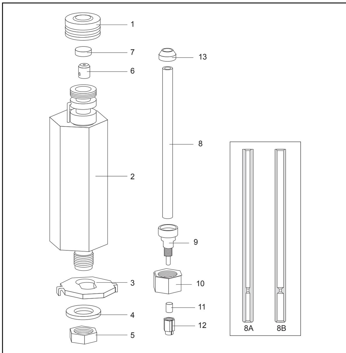
**Table 8-1.** Purged Packed Column Injector parts identification table
