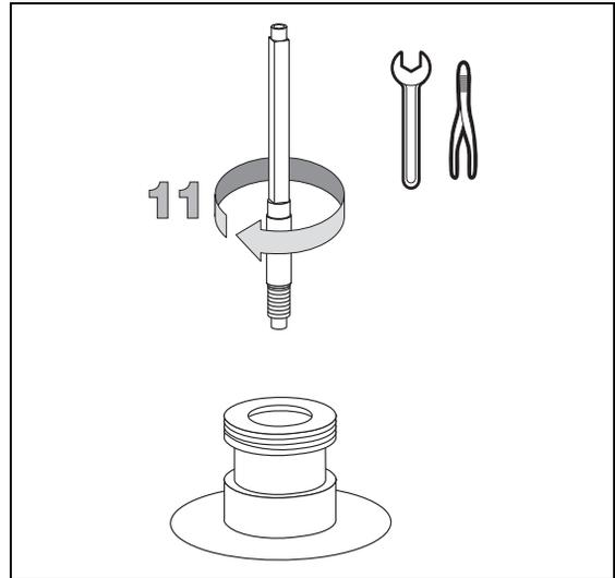
12. Place the detector on its base body, paying attention that the aluminium ring has been inserted in the correct position, then tighten the fixing nut.
