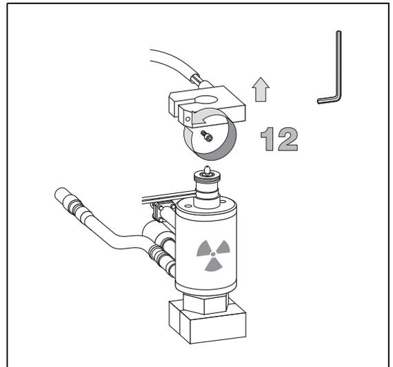
13. Remove the detector adapter unscrewing the two retaining Allen screws. Use a 2.5 mm Allen wrench.
