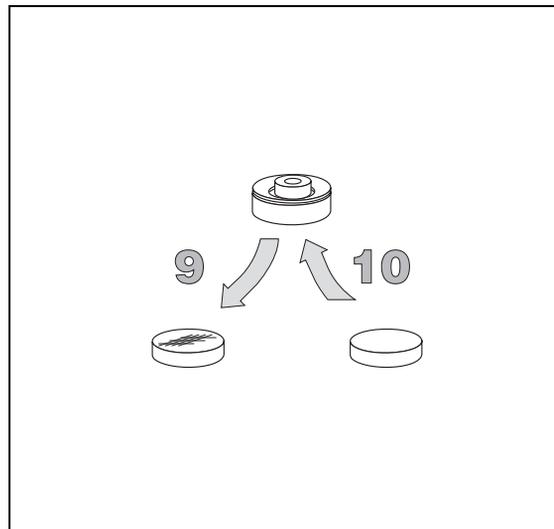
11. Clean the septum support from possible fragments left by the septum and reinsert it into the injector.
