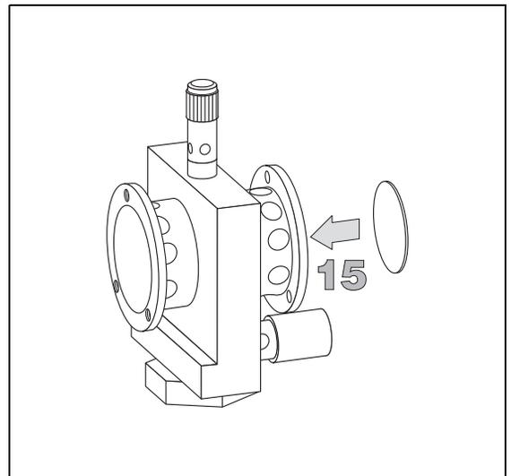
16. Insert the spacer into the flange, letting it stand out for about 5 mm.
