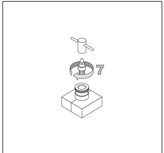
8. Reinsert the detector cell on the detector base body and tighten the fixing screw.
