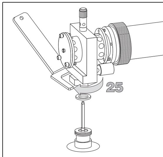
25. Place the detector on its base body, paying attention that the aluminium ring has been inserted in the correct position, then tighten the fixing nut.
