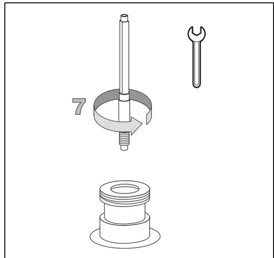
8. Place a new jet into the housing and tighten it.
