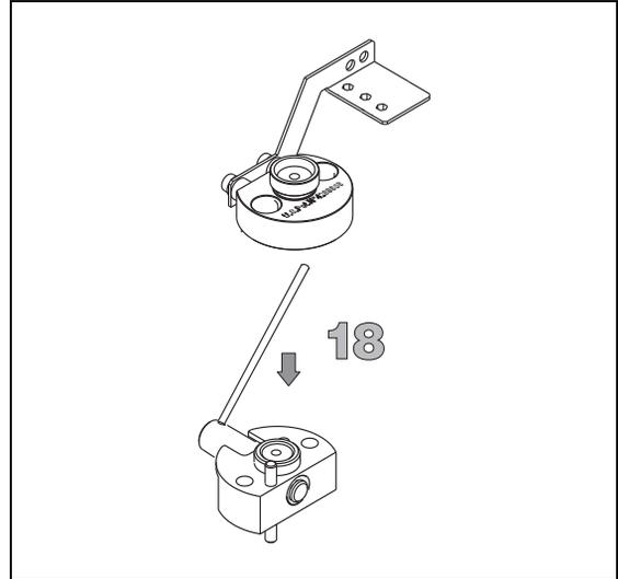
19. Remount the injector body on its base, tightening the two Allen screws.
