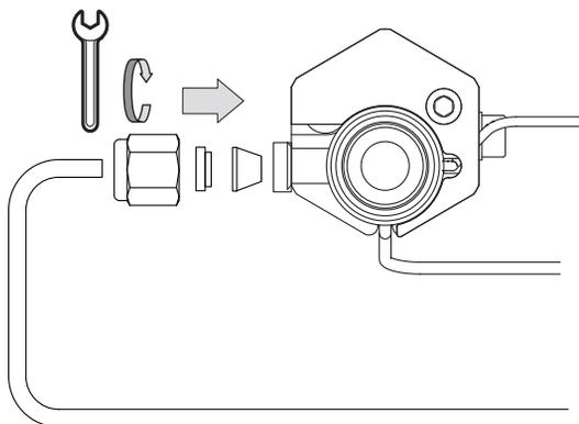
12. Connect the new split line tubing to the split line dummy filter
