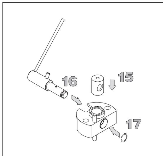
18. Reassemble the two parts of the injector body.
