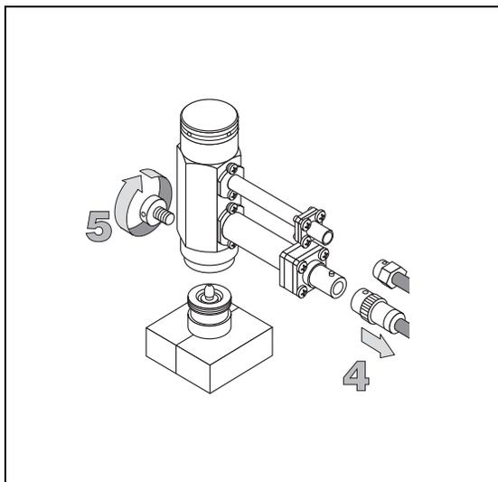
6. Using the tool provided with the GC, unscrew the jet.
