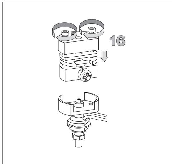
17. Insert the valve lever into its housing, tightening the retaining screw.
