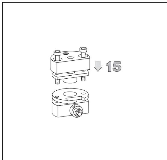
16. Remount the injector body on its base, tightening the two Allen screws.
