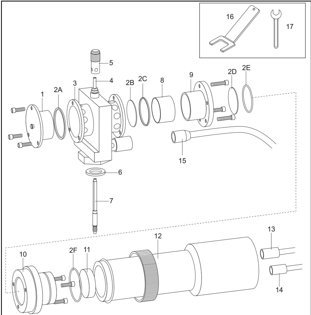
**Table 14-1.** Flame Photometric Detector (FPD) parts identification table
