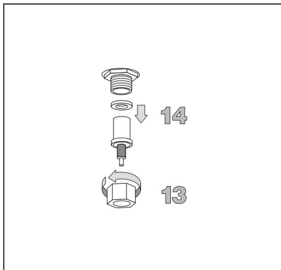
16. Reinsert the silver seal and the terminal fitting.
