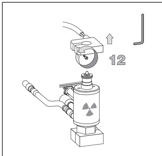
13. Remove the detector adapter unscrewing the two 3 mm Allen screws. Use a 2.5 mm Allen wrench.
