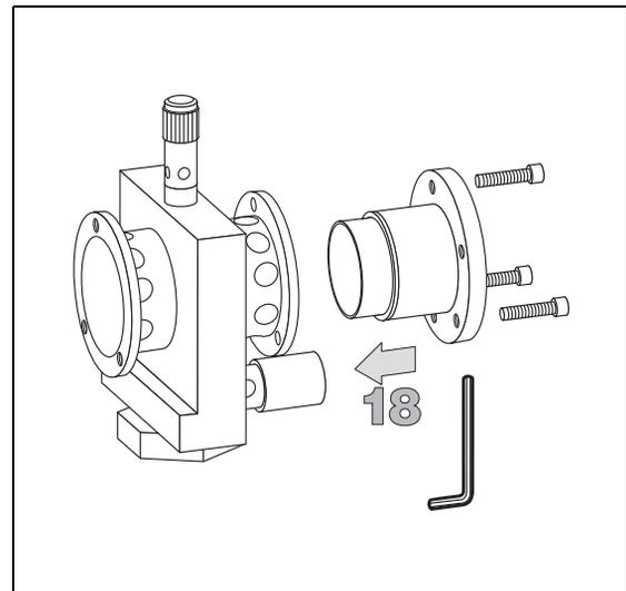
20. Insert the mirror plug in the detector body and fix it with the relevant Allen screws.
