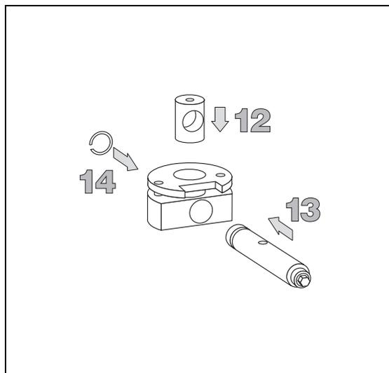
15. Reassemble the two parts of the injector body.
