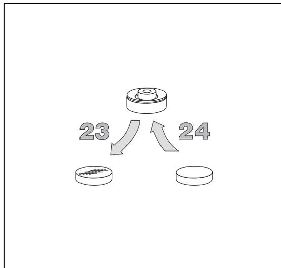
25. Clean the septum support from possible fragments left by the septum and reinsert it into the injector.
