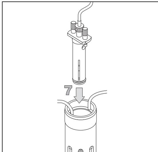
8. Tighten the two knurled screws to fix the lamp holder to its housing.
