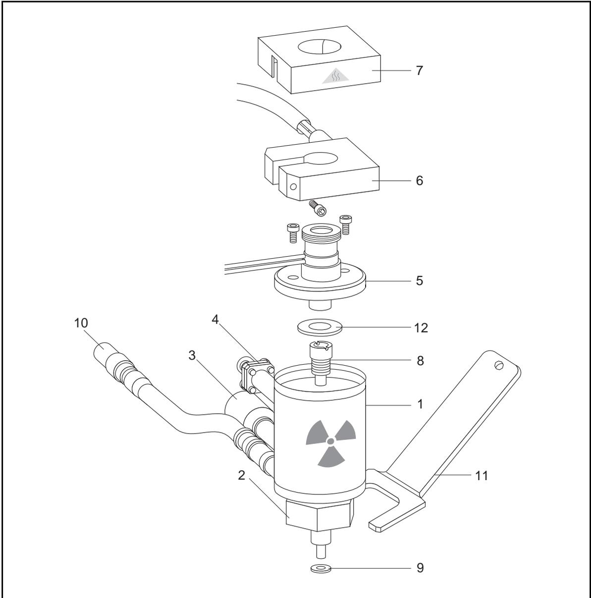
**Table 17-1.** Electron Capture Detector (ECD) parts identification table (Stack configuration version)
