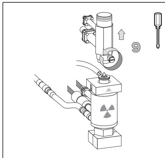
10. Disconnect the signal, excitation and heater cables from the ECD detector
