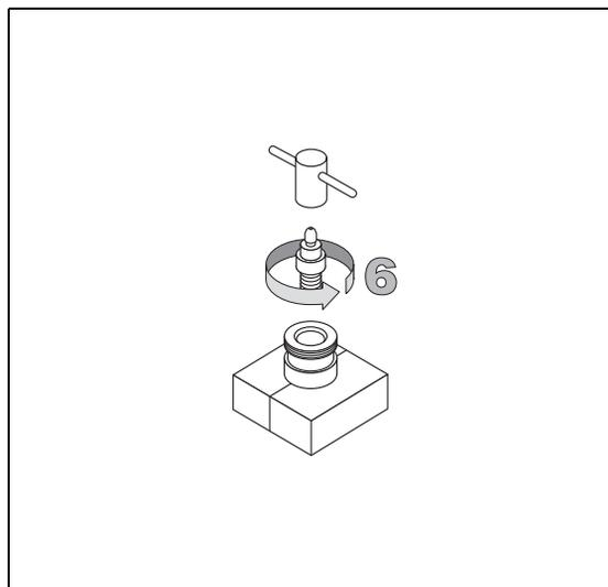
7. Place a new jet into the housing and tighten it with the proper tool. Ensure the jet is perfectly vertically aligned to avoid damaging its ceramic part.
