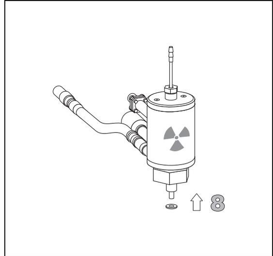
9. Remount the detector on its base body, tightening the fixing nut with the proper tool.
