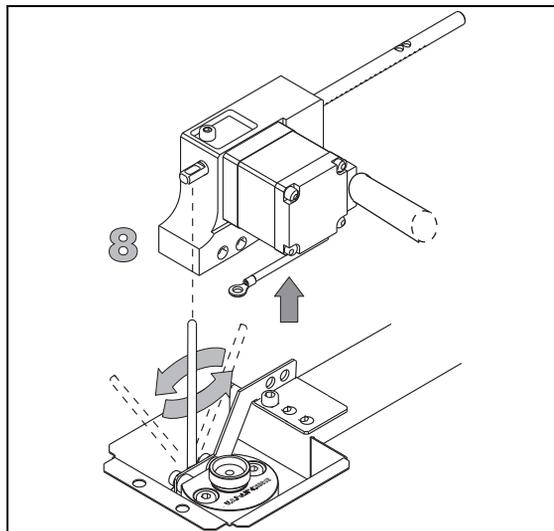
9. Loosen the two screws A on the side of the OC head. Unscrew the remaining fixing screws of the head arm by using a 3-mm Allen wrench.
