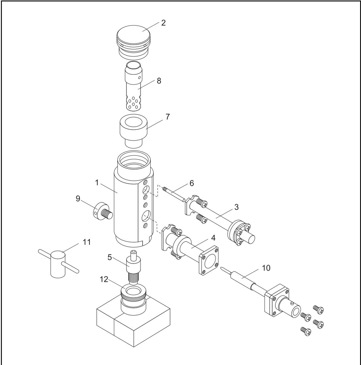
**Table 13-1.** Nitrogen Phosphorus Detector (NPD) parts identification table
