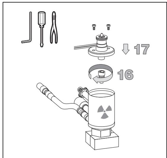
Clean or Replace the Collecting Electrode (NPD on ECD)
