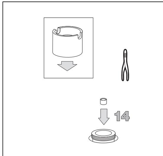
15. Holding a liner with tweezers, place a graphite seal over it, making sure to leave a distance of about 10 mm between the seal and the liner end.
