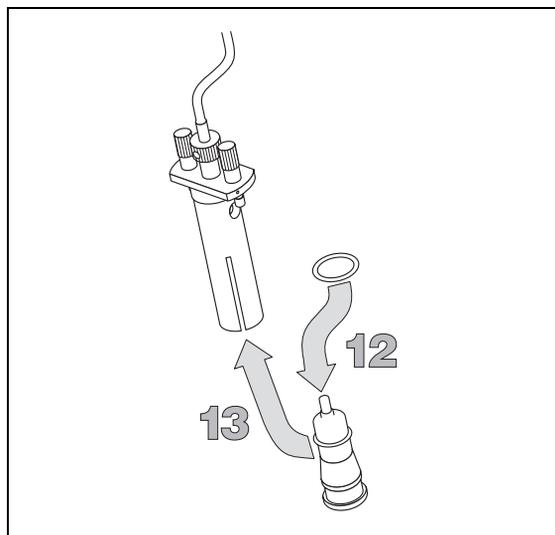
14. Insert the lamp holder into the lamp housing.
