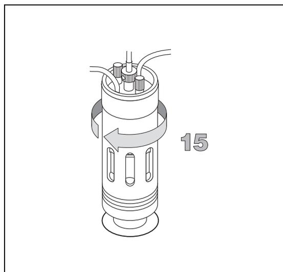
16. If leaks are still detected, loosen the two knurled nuts that fix the lamp holder to the lamp housing.
