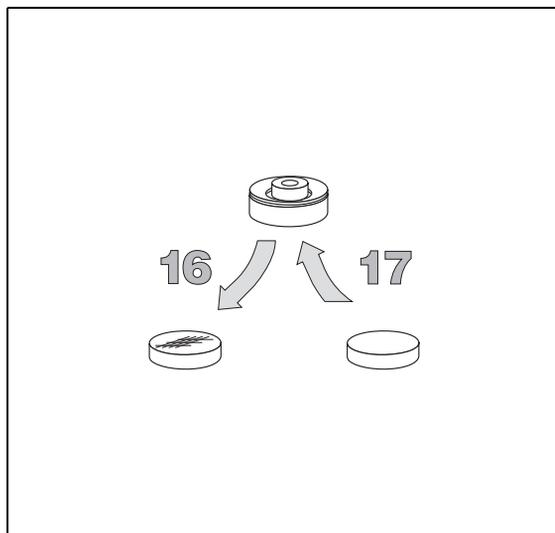
18. Place the septum support into its housing inside the injector.
