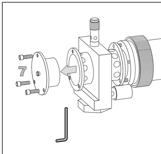
9. Insert the mirror plug in the detector body and fix it with the relevant Allen screws.
