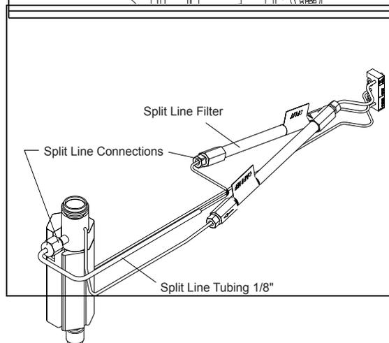
9. Disconnect the split line tubing from the injector body and from the split line filter.
