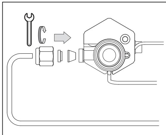
12. Connect the new split line tubing to the split line filter
