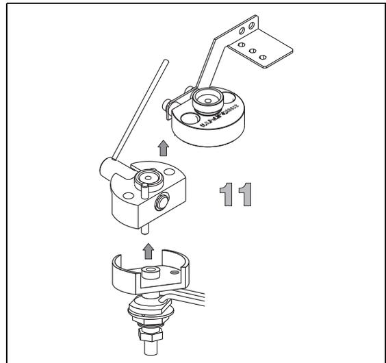
12. Remove the clip that retains the rotary valve.
