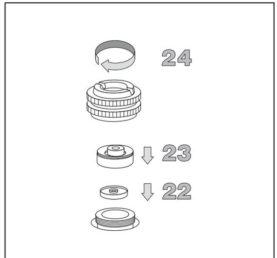
24. Tighten the injector cap to finger tight.
