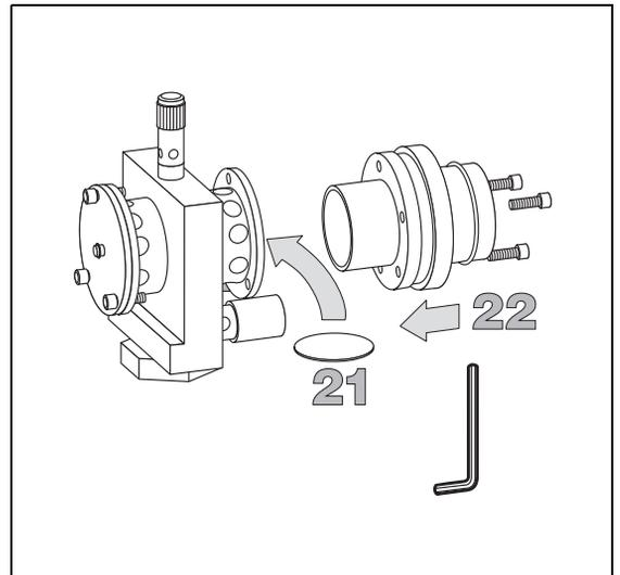
23. Reinsert the filter into the support. The mirror face must be oriented towards the flame
