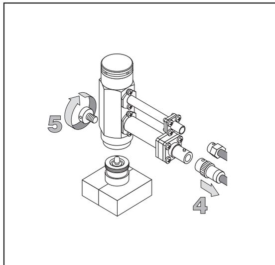
6. Using the tool provided with the GC, unscrew the worn jet from the detector base body.
