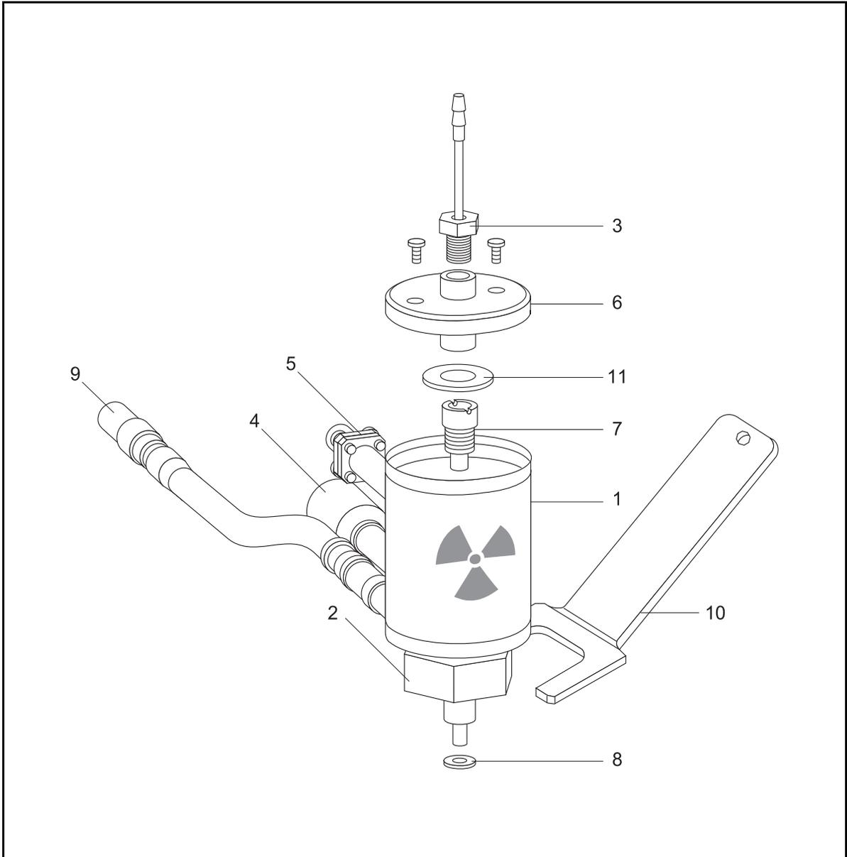
**Table 12-1.** Electron Capture Detector (ECD) parts identification table
