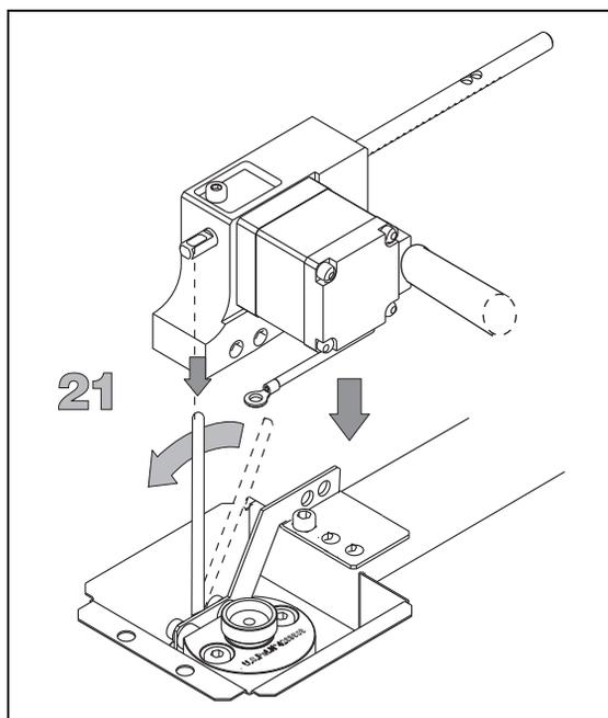
22. Adjust the position of the automatic actuator up to align the fixing holes provided on the actuator body with the corresponding fixing holes located on the fixing arm of the OC head. Fix the parts by using the two fixing screws.
