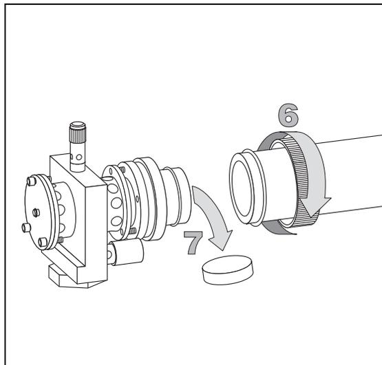
8. Insert the new filter into its housing. The mirror face must be oriented towards the flame.
