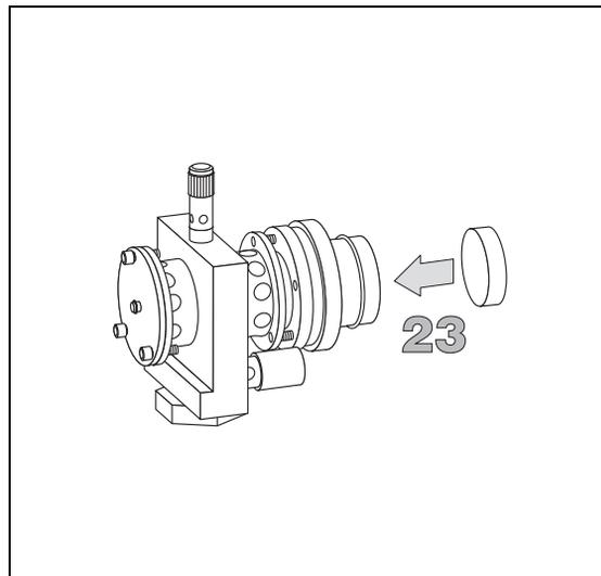
24. Reassembly the photomultiplier tube and the detector body, then fix them together tightening the knurled nut.
