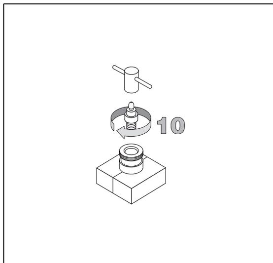
11. Place the detector cell on the detector base body and tighten the fixing screw.
