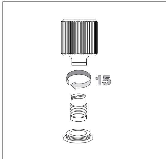
16. Remove the septum from the septum holder using a non-metallic sharp tool.
