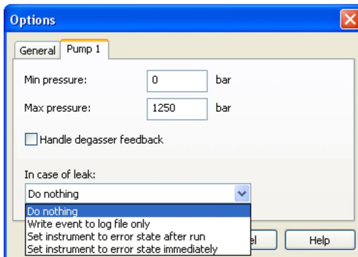
5. Select the action that you want the pump to take when the leak sensor detects a leak.
