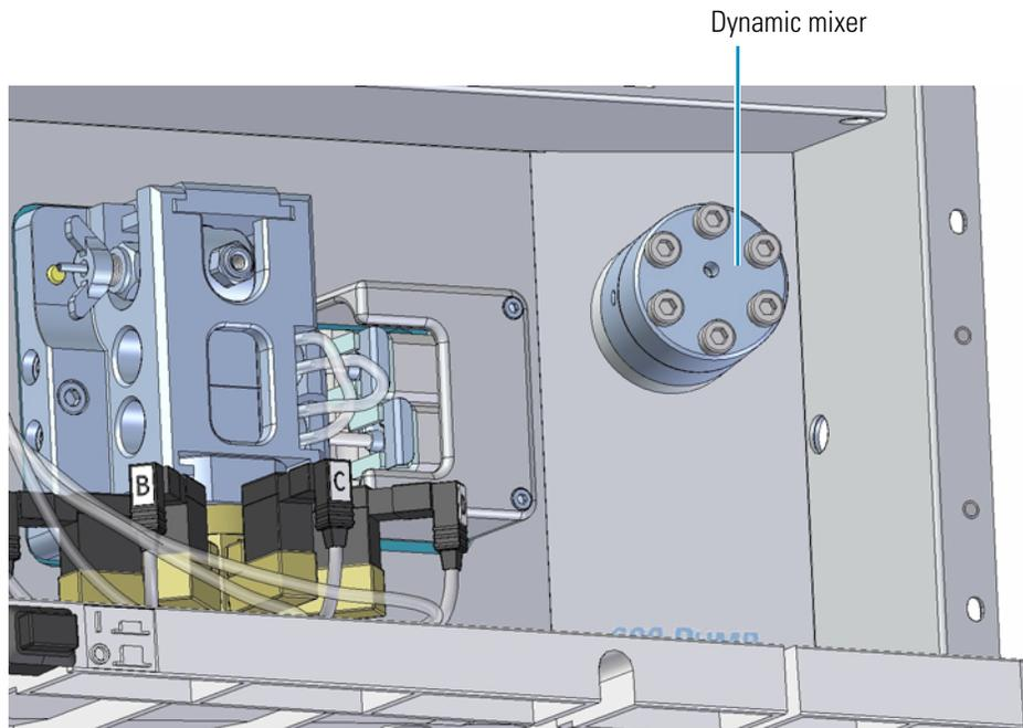
5. From the back side of the front panel (see [Figure 31](#)), secure the dynamic mixer with the screws that you removed in [step 1](#) on [page 37](#).
