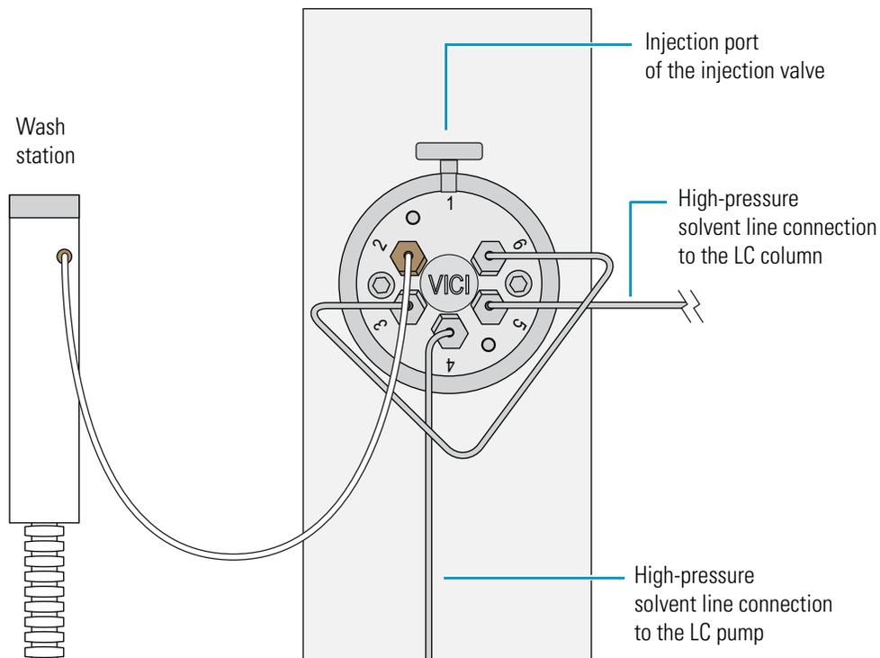
3. Using a 1/4 in. open-end wrench, tighten the fitting.
