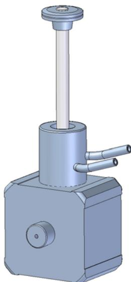
11. Remove the guide bushing/piston assembly from the displacement chamber (see [Figure 101](#)).
