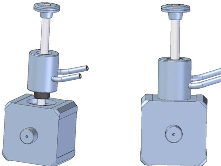
10. Hold down the guide bushing and slide the piston up until it is out of the seal (see [Figure 100](#)).
