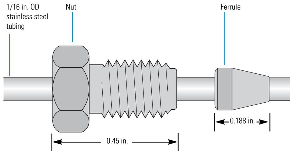
3. Using a 1/4 in. open-ended wrench, tighten the nut.
