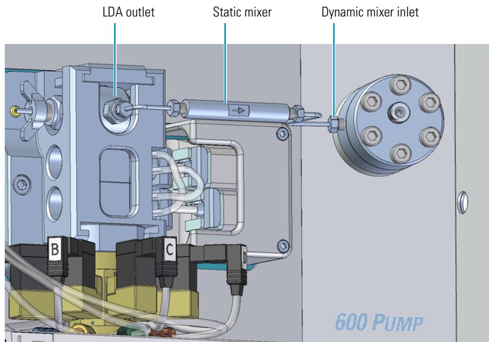
2. Connect the outlet of the dynamic mixer to the autosampler inlet (see [“Connecting the Solvent Line Between the Pump and the Autosampler”](#) on page 27).
