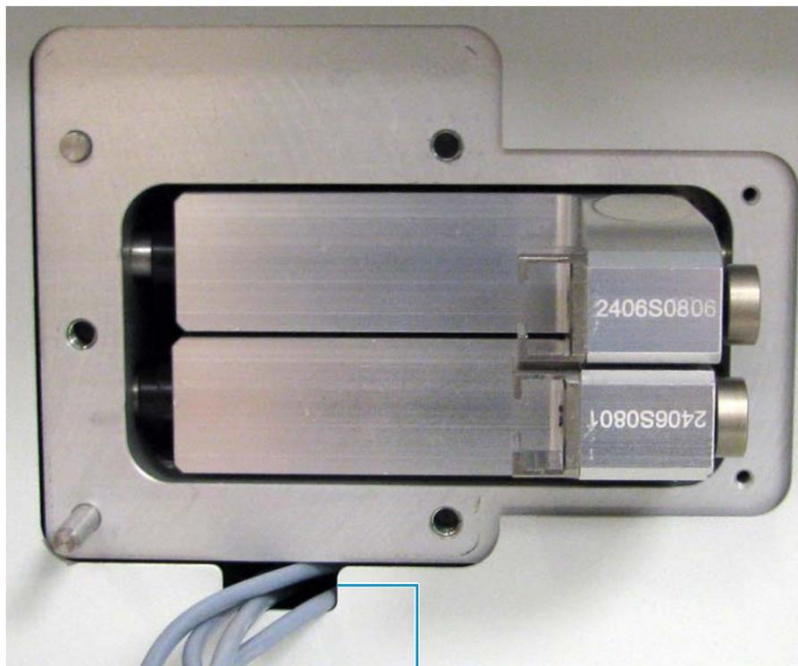
Slot for the proportioning valve cables
