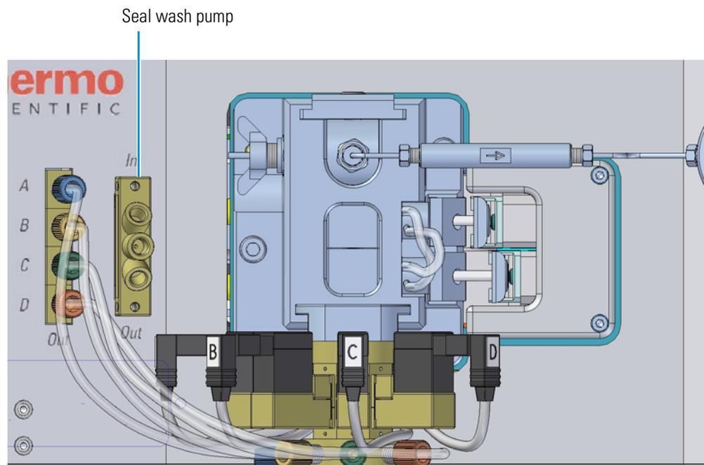
5. Using the two screws that you removed in [step 3](#) on [page 44](#), secure the seal wash pump to the front panel of the pump (see [Figure 38](#)).
