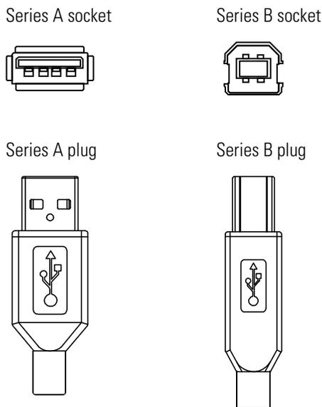
2. Connect the series B plug (see [Figure 7](#)) of the USB cable to the USB port on the back of the Accela pump.
