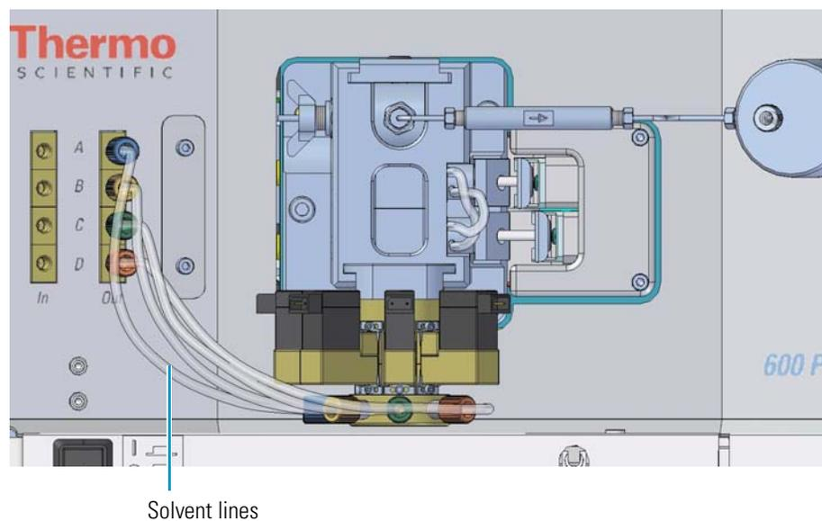
**Figure 67.** Pump with the solvent lines disconnected
