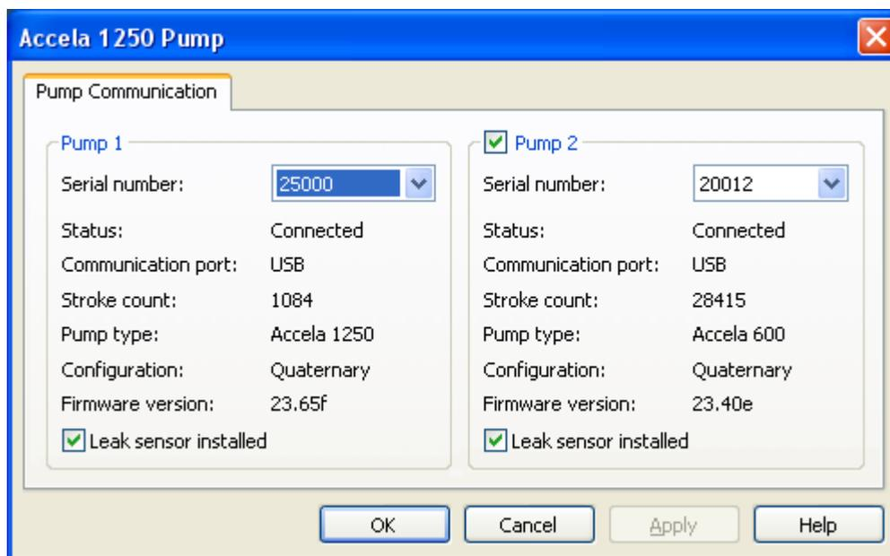
6. Ensure that the Serial Number list displays the pump's serial number and that the Status readback displays Connected.
