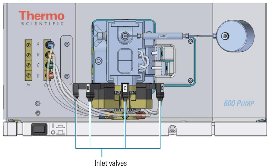
3. Disconnect all four solvent lines from the inlet module (see [Figure 66](#) and [Figure 67](#)).
