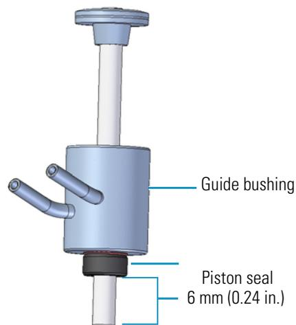
9. Insert the piston into the bore of the displacement chamber. Do not apply any side load onto the seal during this process (see [Figure 99](#)).
