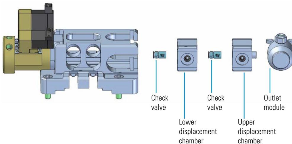
3. Insert the lower displacement chamber into the main body of the LDA.
