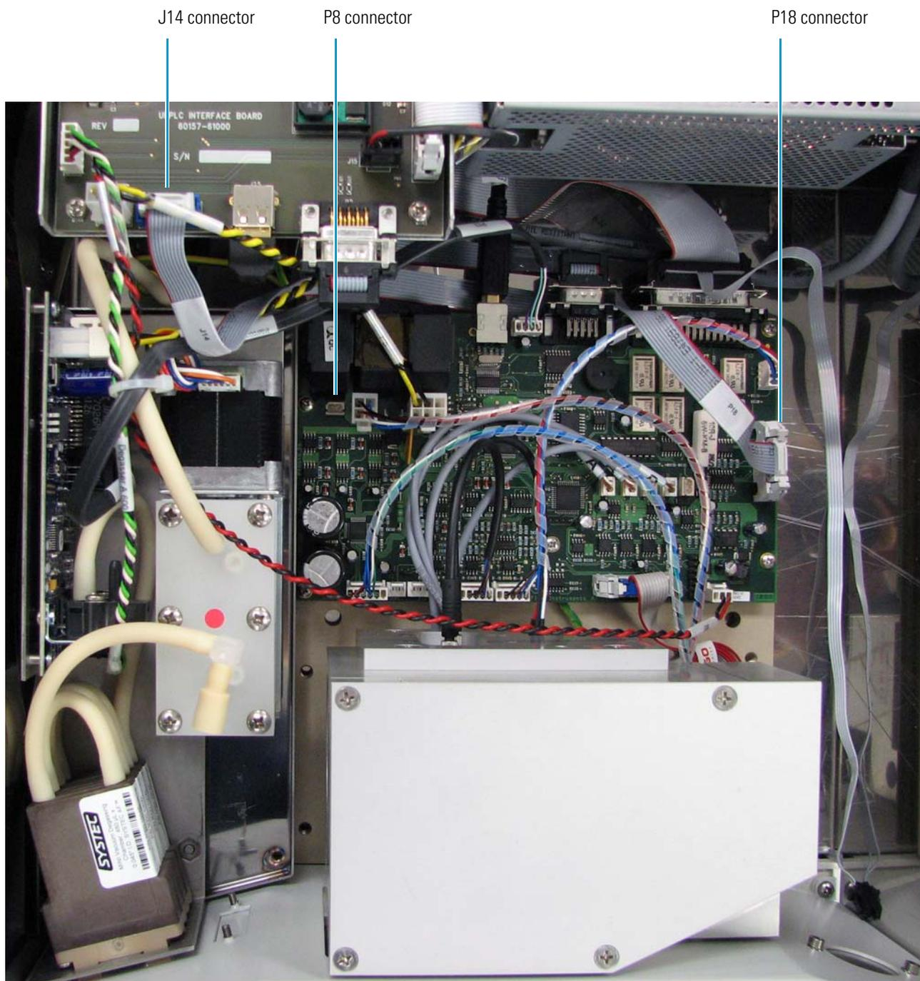
7. Connect the new cable (see [Figure 44](#)) to the J14 connector on the Interface board and the P18 and P8 connectors on the Controller board.
