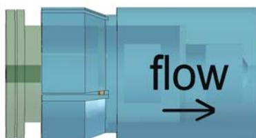
**Figure 81.** Inserting the displacement chambers, check valves, and outlet module into the LDA
