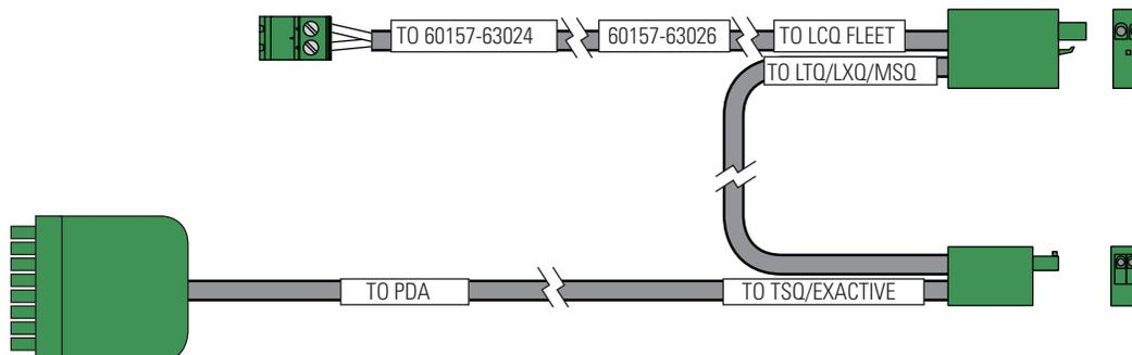
❖ **To connect the contact closure cables to the Accela LC system modules**
