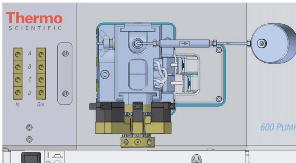
4. Using a 1/4 in. open-end wrench, unscrew the static mixer at the outlet of the LDA and at the inlet of the outlet module (see [Figure 68](#)).
