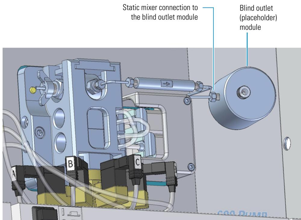
4. If the high-pressure tubing is connected between the pump and the autosampler, using a 1/4 in. open-end wrench, disconnect the high-pressure solvent line from the blind outlet module.
