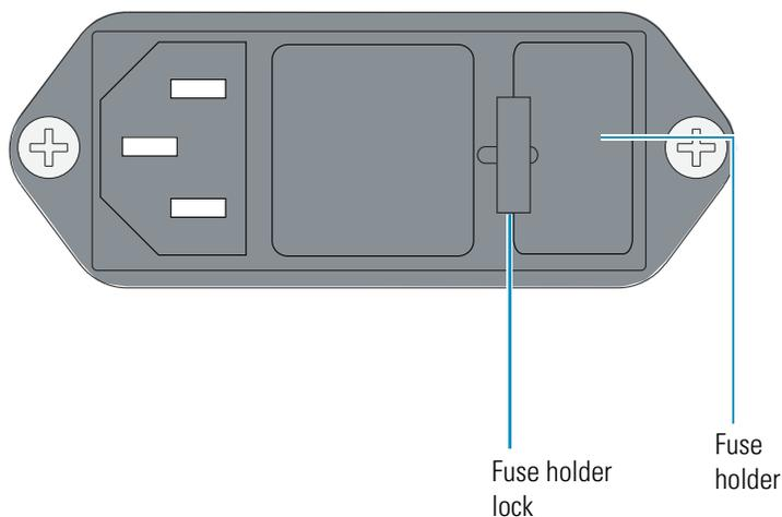
3. Remove the fuses and replace with the appropriate fuses.
