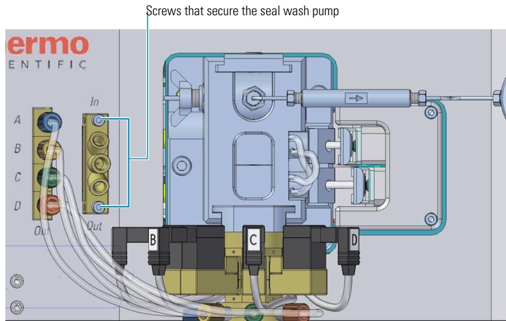
6. Using a 2.5 mm hex ball driver, tighten the screws.
