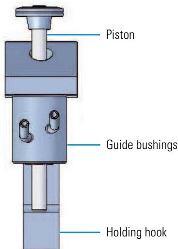
4. Insert the piston into the primary seal no more than 3 mm (0.12 in.) (see [Figure 97](#)). The primary seal is located inside the displacement chamber.
