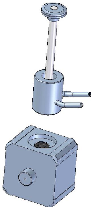
12. Repeat [step 3](#) through [step 11](#) to replace the primary piston seal of the second displacement chamber with a new piston seal.
