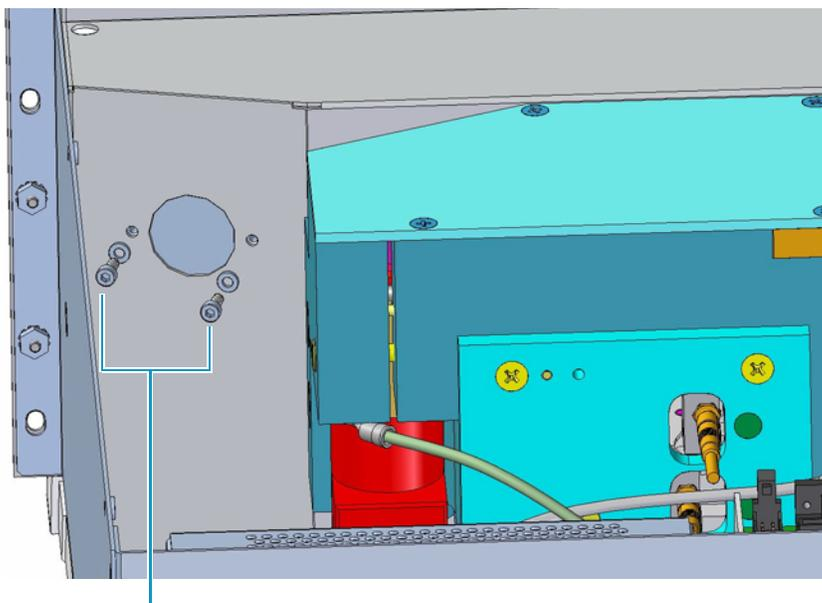
Screws that secure the blind outlet (placeholder) module to the front panel of the pump
