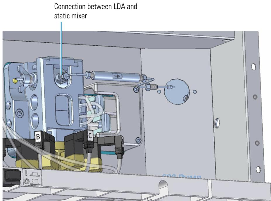
**Figure 29.** Static mixer disconnected from the pump
