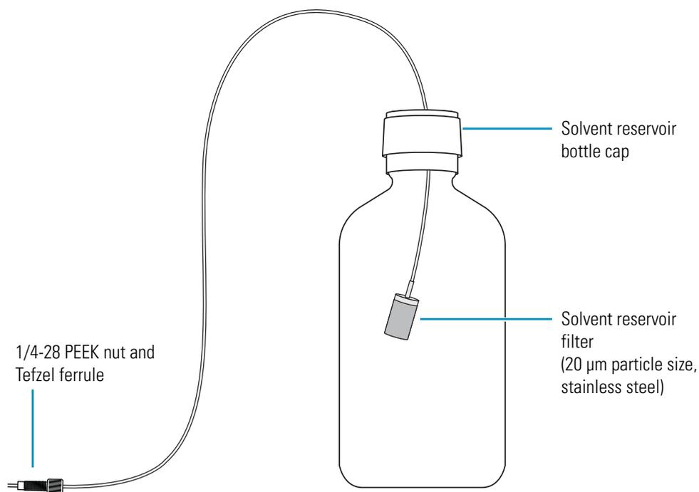
4. Insert the solvent reservoir filter and inlet line into one of the solvent reservoir bottles, and screw the cap onto the solvent reservoir bottle until it is secure.
