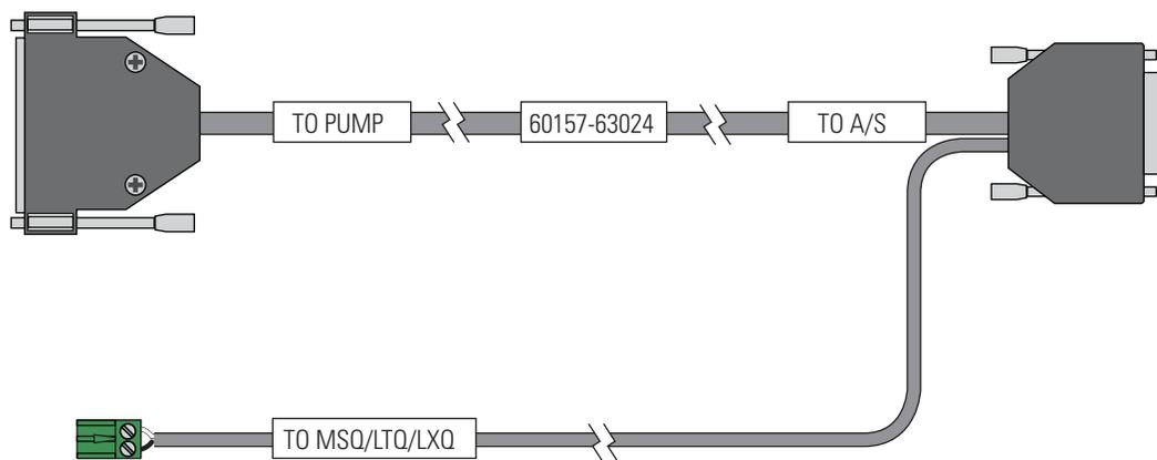
Figure 11 shows the adapter cable for an Accela LC system with an Accela Open Autosampler and an Accela detector (refractive index, UV/Vis, or photodiode array detector) or TSQ Series or Exactive mass spectrometer.
