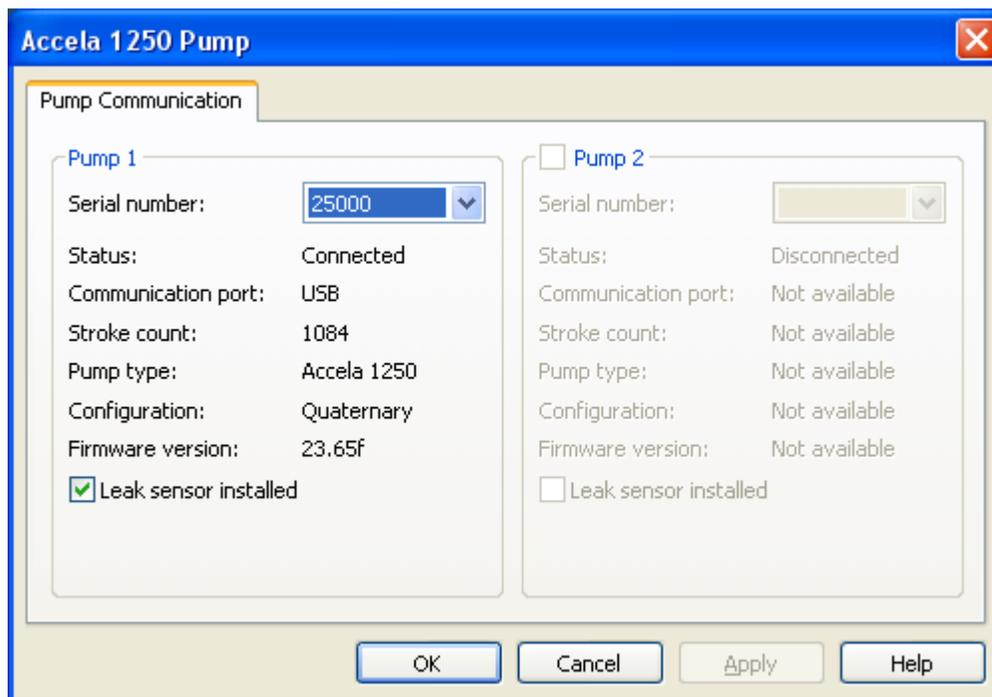
8. If your Accela pump has a leak sensor, select the **Leak Sensor Installed** check box.
