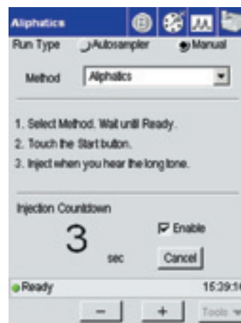
The injection countdown ensures high precision for manual sample injections.
